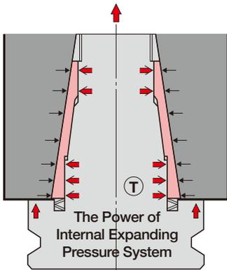
1. When **3LOCK** tool is inserted into **3LOCK** spindle (before clamping), the gap between the spindle flange and the tool flange is ; #40 : 0.2mm, #50 : 0.5mm
