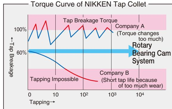
■ The torque of CCW is 1.4 times of the torque of CW to prevent the problem of the swarf.
