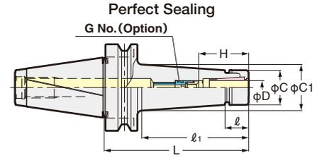
When SK J type nut is used, the total chuck length will be extended by 6mm. **PAT.**
