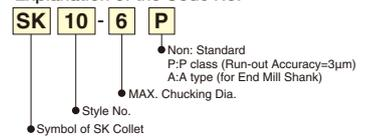
**SK** "A" type SK collet (for End Mill Shank) are marked  . The acceptable shank tolerance is h8. Code No. is e.g. SK10-10A
