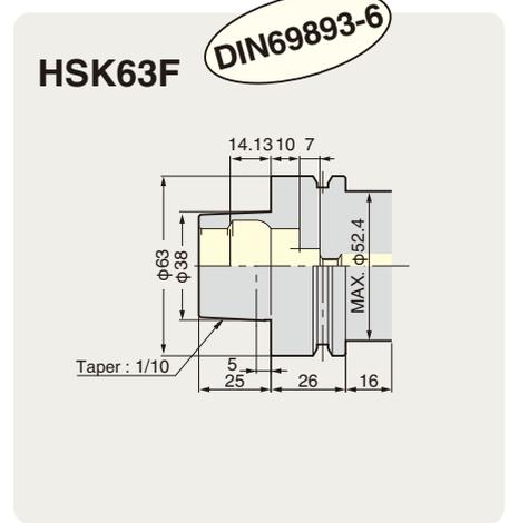
NIKKEN HSK Tooling has a hole and a flat for mass balancing as standard. Hole for manual clamp and hole for ID are not standardized. Special HSK\_A type which U grooves and drive key slots are symmetric design without V notch is also available. Please contact with us.
