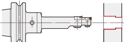
Please specify each boring dia., depth, and necessary length from the gauge line.
