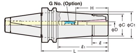
High Speed 3LOCK tooling (MBT) can be used as the triple contact tooling on the M/C where spindle is BT double face contact system. PAT.
