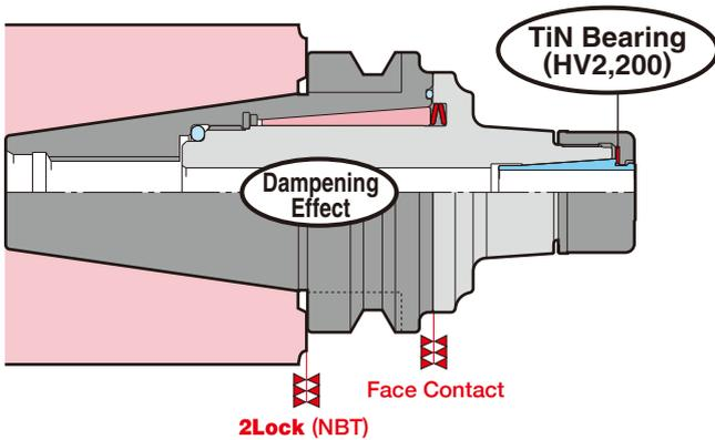
Slim Collet with 8 degree taper to satisfy the accuracy and the high gripping torque.
