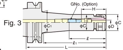
When SK J type nut is used, the total chuck length will be extended by 6mm.
