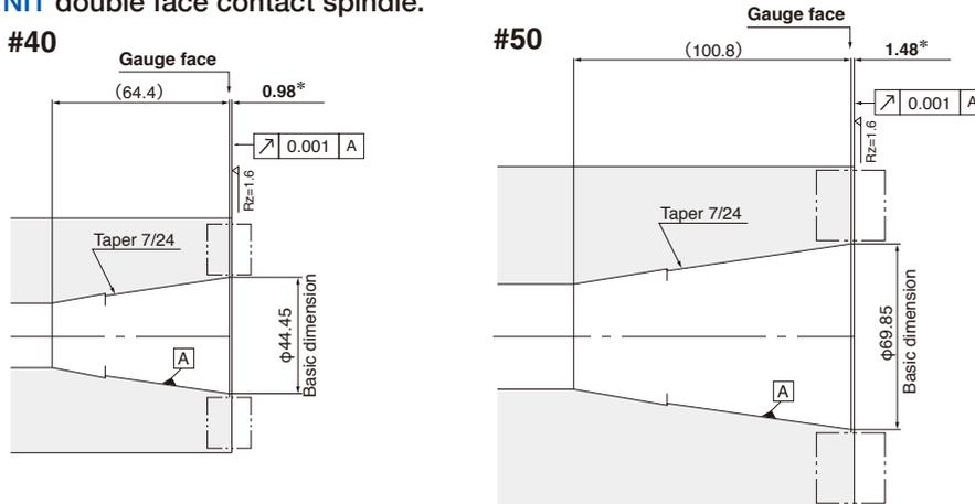
\* mark: The tolerances of the extension of the spindle flange from gauge face depend on the M/C.
