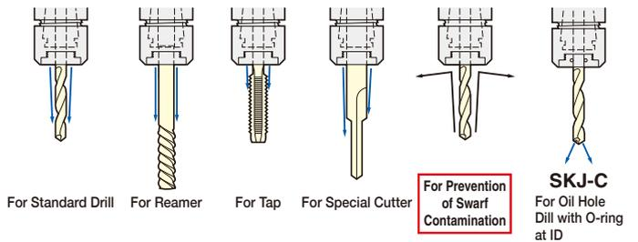
When SK J type nut is used, the total chuck length will be extended by 6mm.
