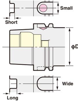
HSK A shank is based on ISO12164-1 (DIN69893-1) and Hollow Shank Taper with 1/10 Taper and Double Contact System of Taper & Flange. Its dimension is unsymmetrical shape such as;
