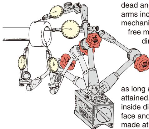
Free flexing with single knob, no dead angle and long reach, two arms incorporating ball joint mechanism at both ends provide free movement in any direction such as vertical, lateral, longitudinal or rotational etc. If stretched horizontally, a reach as long as **300mm** can be attained. Measurements of inside dia., outside dia., end face and back face etc, can be made at will.
