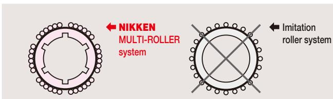
The larger quantity of needle rollers enables the moving of the same load with a small force and less damage on the bearing surface, thus providing a stronger chucking torque without creating even rolling when tightening.
