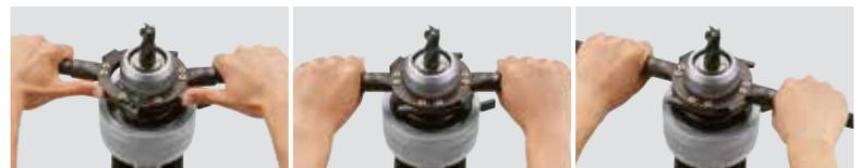
3 easy steps make it possible to clamp, unclamp milling chuck very safely and easily.
