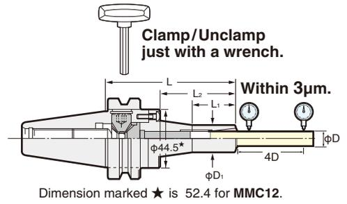
**2LOCK** tooling (NBT) can be used as the double face contact tooling on the M/C where spindle is BT double face contact system.
