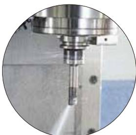
Current developments in inserts (coated TiAlN & CBN) and their improved capability for high speed cutting is remarkable. However, the results are based on using these inserts with high-speed cutting conditions (their performance is reduced when used for medium or low cutting speeds). The ZMAC Boring Head has been designed to optimise this new high-speed cutting technology.
