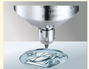
The die mould profiling by the φ0.2mm end mill at the 150,000min<sup>-1</sup> can be done continuously and stably.
