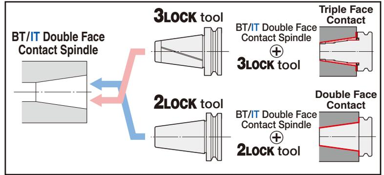
**2LOCK** tool can also be used on the machine with BT/IT standard spindle.
