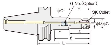
When SK J type nut is used, the total chuck length will be extended by 6mm. PAT.
