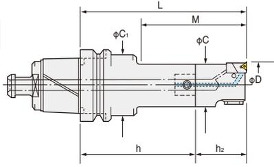
No Micro Vibration due to Double-Contact Support of Cartridge. Long Tool-Life & High Accuracy.
