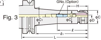
**2LOCK** tooling (NBT) can be used as the double face contact tooling on the M/C where spindle is BT double face contact system.
