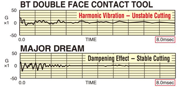
**Difference due to Dampening Technique and Effect**
