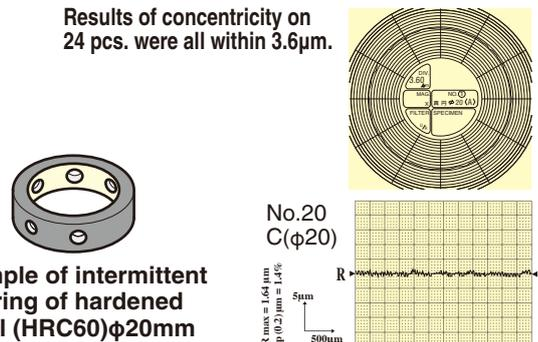
Example of intermittent boring of hardened steel (HRC60)φ20mm
