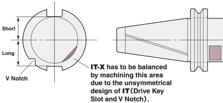
MIT Shank is **3LOCK SYSTEM** for IT shank. IT shank is based on ISO 7388/1-'83 (DIN69871-'90) and its flange has an unsymmetrical shape.
