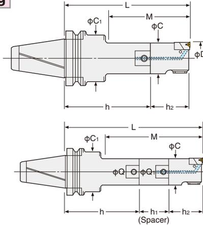
No Micro Vibration due to Double-Contact Support of Cartridge. Long Tool-Life & High Accuracy.
