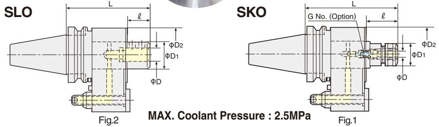
Oil Mist type holder which is not necessary to use coolant is also available for health and safety environment regulation. Please contact with us. e.g. **BT40-SLO25M-130**
