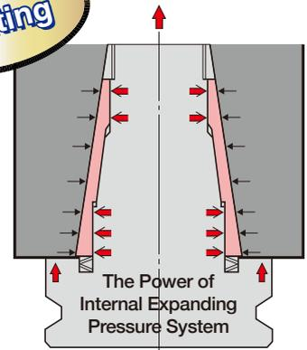
Machine spindle expansion due to the centrifugal force at the high speed rotation or heat expansion
