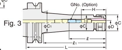
When SK J type nut is used, the total chuck length will be extended by 6mm.
