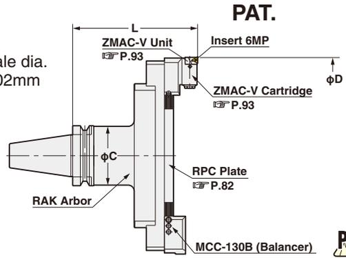
Boring Dia:  $\phi 130 \sim 595\text{mm}$  for Finishing.
