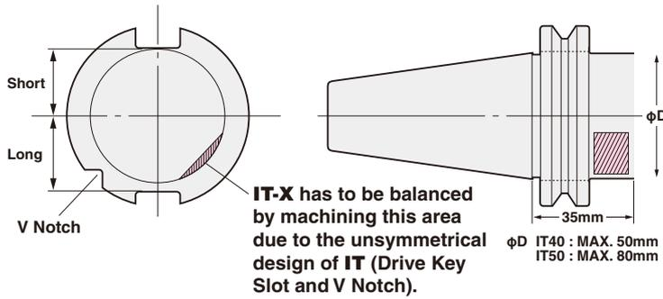
IT shank is based on ISO 7388/1-'83 (DIN69871-'90) and its flange has an unsymmetrical shape.
