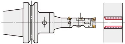
Please specify the boring dia., depth, and necessary length from the gauge line.
