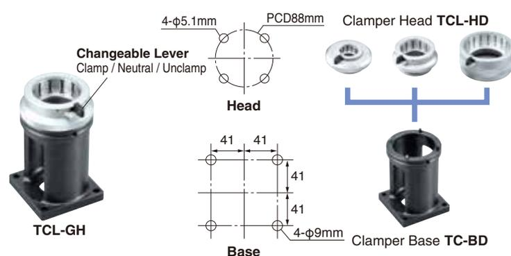
TCL-GH clamper is designed for symmetrical holders without drive key slots or U-groove. The TCL-GH clamper is also suitable for the other shank tooling with same flange diameter as E & F type. e.g. TCL-GH63 is suitable for HSK63A, 63E, 63F, BT40 and NC5-63. By changing the clamper heads to the suitable sizes, the same TCL-BD base can be used for the other sizes of shank.
