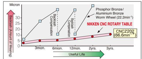
\* Rotation speed of motor = 3,000min<sup>-1</sup>
