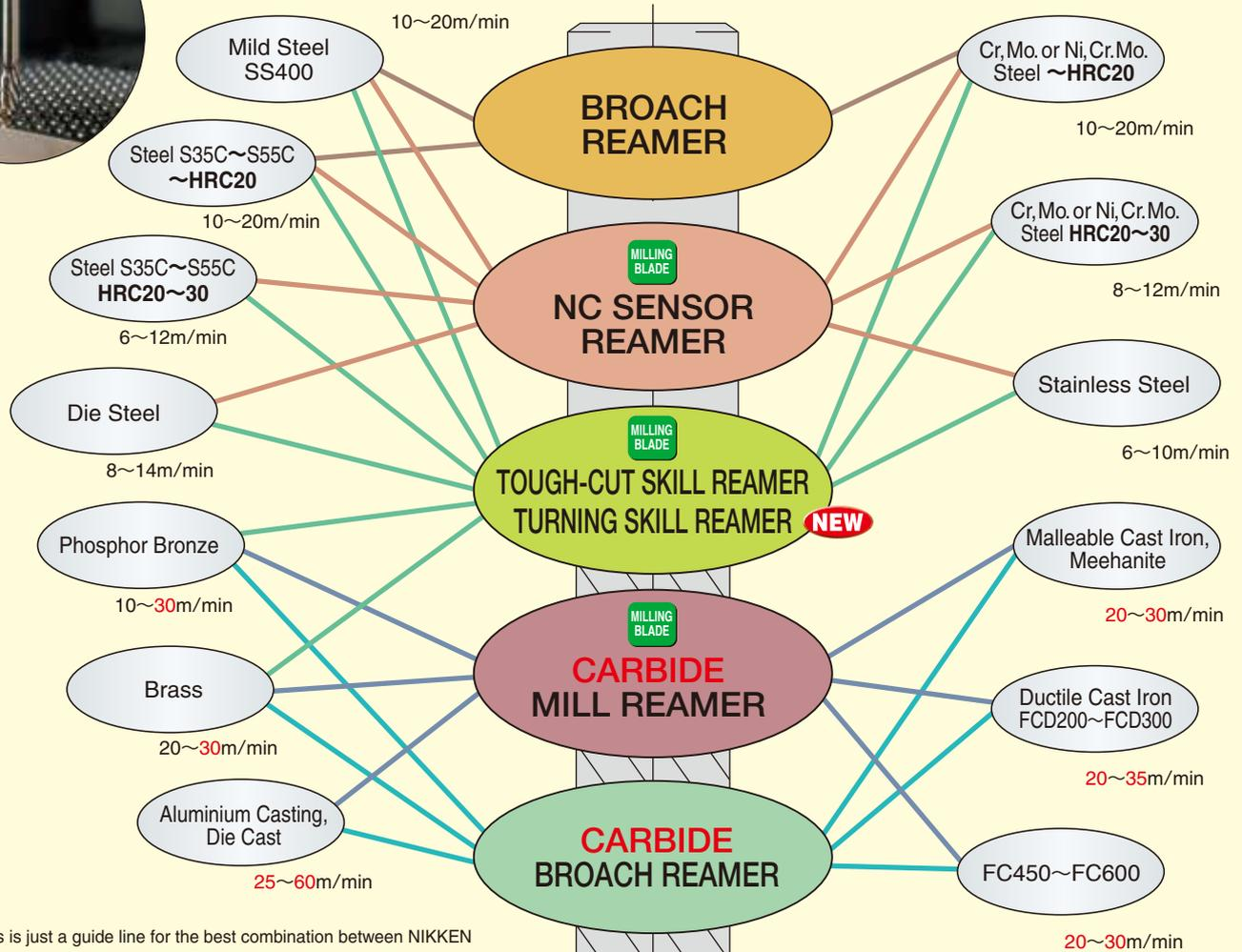
This is just a guide line for the best combination between NIKKEN reamers and each material, Therefore Broach reamer also can be used on die steel or non-alloy steel.
