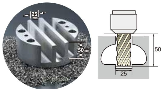
**Material: Ti6Al4V Titanium 25mm, 6teeth Carbide Roughing End Mill 25 X Depth 50mm 1 Path Milling Never Pull-Out**
