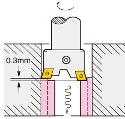
Approx. double removal of below cutting condition is possible by **-0.3 Cartridge**.
