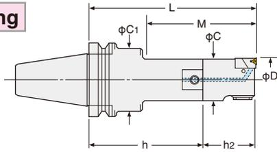
No Micro Vibration due to Double-Contact Support of Cartridge. Long Tool-Life & High Accuracy.
