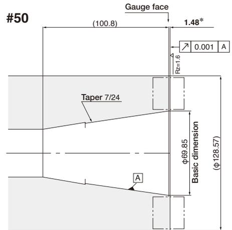
\* **mark**: The tolerances of the extension of the spindle flange from gauge face depend on the M/C.
