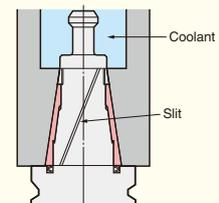
Coolant can not be sealed at taper connection for **3LOCK** tooling. Please **2LOCK** tooling instead.
