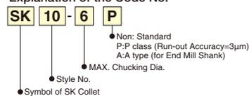
**SK** "A" type SK collet (for End Mill Shank) are marked **P**. The acceptable shank tolerance is h8. Code No. is e.g. SK10-10A
