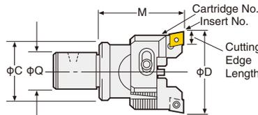
For Heavy Duty Boring of Iron and Cast Iron
