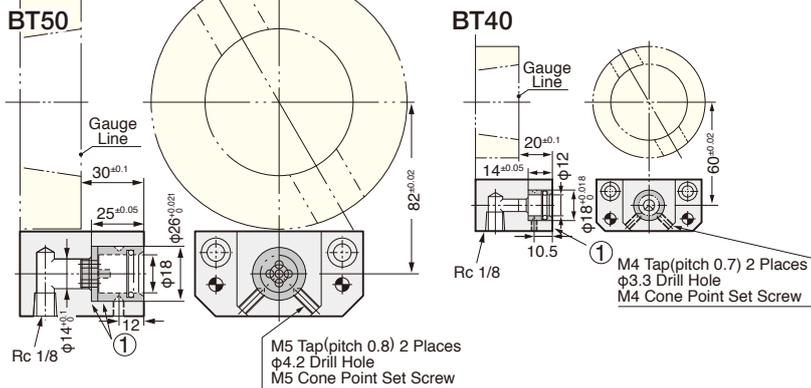
1. Please use **NIKKEN Bushing & Push Pin for the Oil Hole Holder ①** and make the Stopper Block by yourself.
