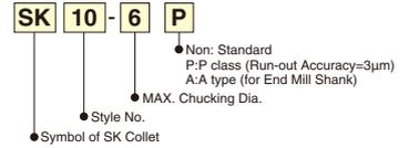
**SK** "A" type SK collet (for End Mill Shank) are marked **P**. The acceptable shank tolerance is  $h_8$ . Code No. is e.g. SK10-10A
