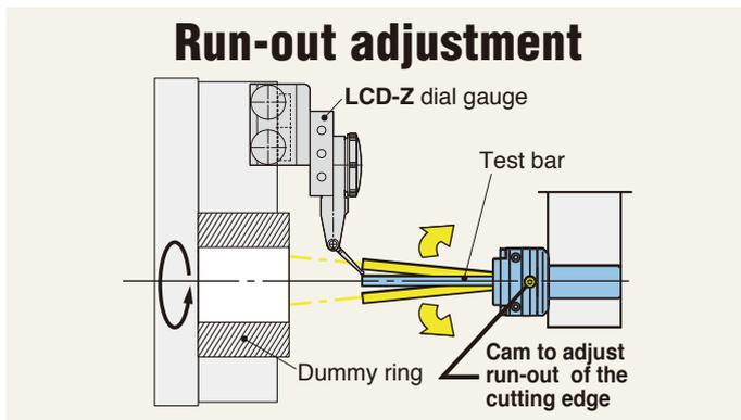
Run-out adjustment range at the tip of 100mm test bar : 0.05mm
