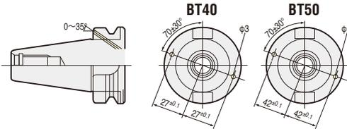
NISHIDA **BT40** Machine's Flange Through Hole alignment is unique. Option **(T)** is available. Specify as **BT40-C20T-90**
