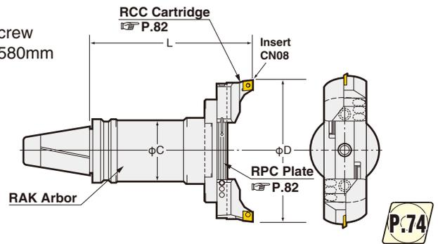
Boring Dia:  $\phi 130 \sim 580\text{mm}$  for Roughing.
