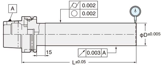
Exact size of  $\phi D$  and  $L$  are marked on each test bar.
