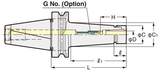
High Speed **3LOCK** tooling (MBT) can be used as the triple contact tooling on the M/C where spindle is BT double face contact system.
