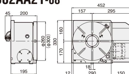
Pneumatic Clamping Torque UP 588Nm
