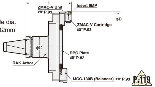
Boring Dia:  $\phi 130 \sim 595\text{mm}$  for Finishing.
