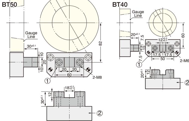
1. Please use **NIKKEN Original Stopper Block for Spindle Speeder ①** and make the **Stopper Block Base ②** by yourself.
