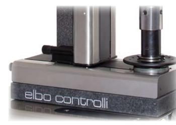
Base and column made of ground granite. The thermal inertia of this material allows the machine to be placed directly in the shop.
