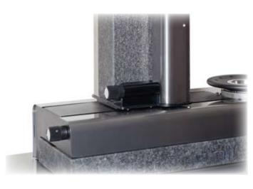
Micrometric registration of X and Z axes by means of two wheels which are essential for the collimation of the measure both with a fixed target function and in self-collimation.
