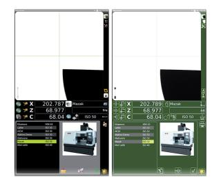
The new software provided the operator the choice of two different graphical layouts: the first provides icons similar to ISO 7000 and the second allows the familiar 'ELBO CONTROLLI' graphical interface.
