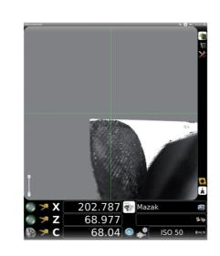
The new software also includes automatic recognition of the spindle via SP-ID (Spindle Identification System). This system allows the presetter to *identify each spindle cartridge as it is* loaded and suggest the correct machine origins, whenever the spindle is changed.
