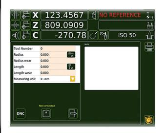
Also included is DNC connection software that allows the transfer of the tool offset data directly into the tool table of the Numerical Control (depending on CNC controller capability).
