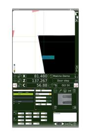
Also included for the first time is the capability for *multi-measurement directly* on the screen. So during tool inspection it is possible to make more than one measurement at a time on the same tool profile.
