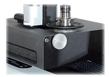
Micrometric movement of the axes are made, for the X axis with two wheels on the right and left of the machine, for the Z axis with one placed at the base of the column. This precise micrometric adjustment is indispensable for the final collimation of the cutting edge of the tools.
